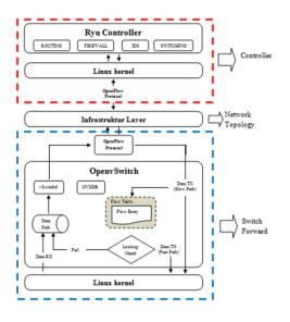
Figure 3 SDN Software Architecture
