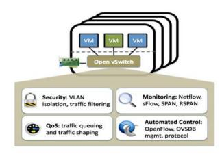
Figure 1 OpenvSwitch Architecture
